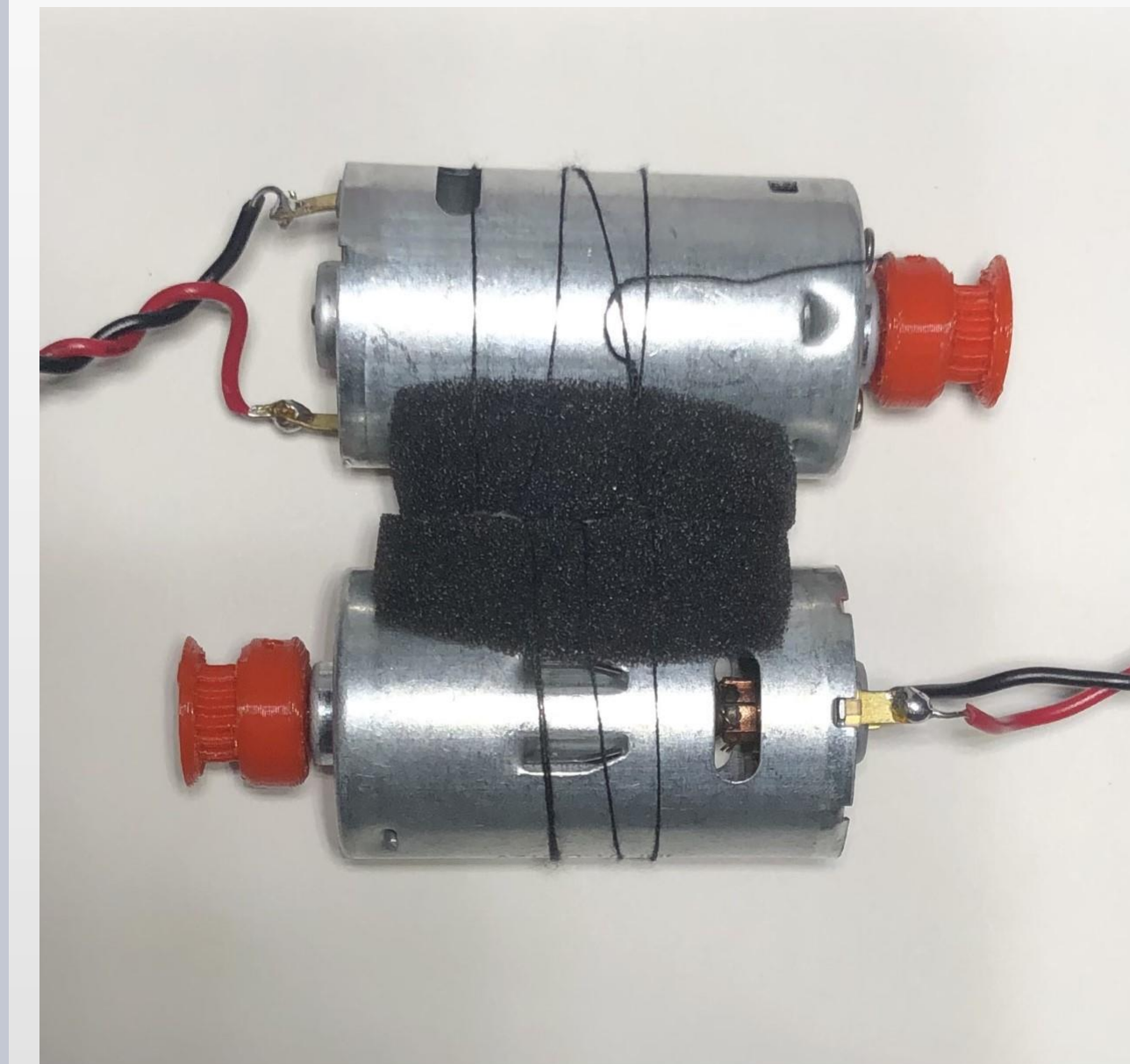
Two DC motor with sheaves and wire connections (Primary mechanical Component of Sewer Scout)
